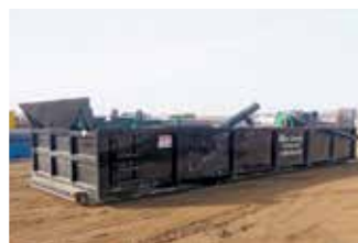
Invert Recovery Automated Shale Bin
